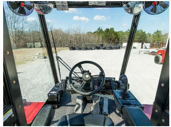
Climate Controlled 2-door Cab - All Steel - Heat, A/C & Defrost (Standard)
